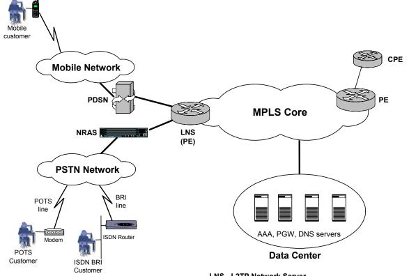
LNS - L2TP Network Server PDSN - Packet Data Serving Node PGW - Packet Gateway (used with SS7 signalling)
