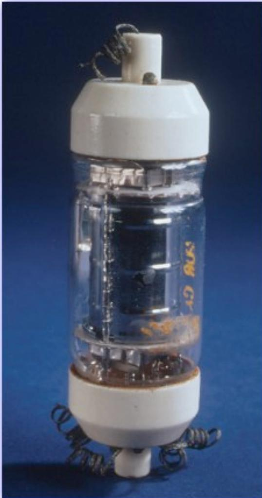
In the 1950s new technology put cables ahead of radio. Small vacuum tubes that could operate under water for 20 years or more meant that amplifiers could be buried at sea with the cable. This boosted the cable's information capacity to the point that it could even carry telephone signals.
