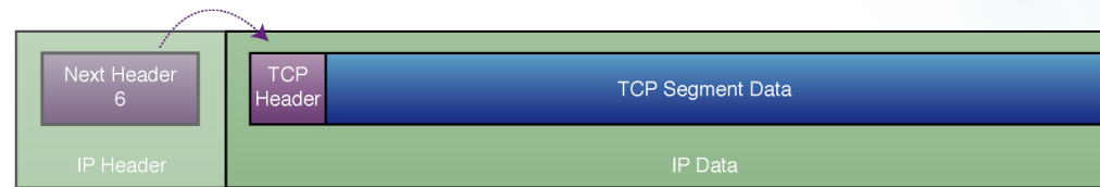
IPv6 Datagram With No Extension Headers Carrying TCP Segment
