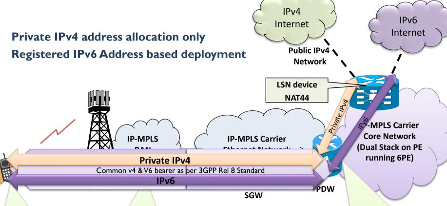
IPv4 & IPv6 user plane with 3GPP defined tunneling:
