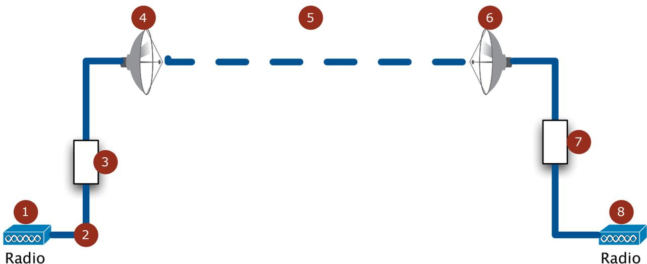
1. The radio takes our energy and modulates it to carry information, we know the output from the radio in Watts, milliWatts, dBw or dBm.
